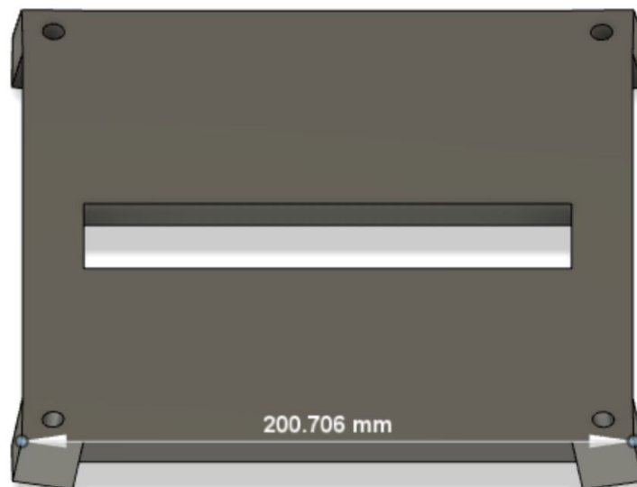
Figure 1: Platform used to mount rigid arm to driving motor and house electronics.
